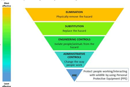
The Hierarchy of Controls is a standard tool applied in occupational safety and health practices to minimize exposure to hazards by implementing effective control solutions. (Credit: CDC.)
